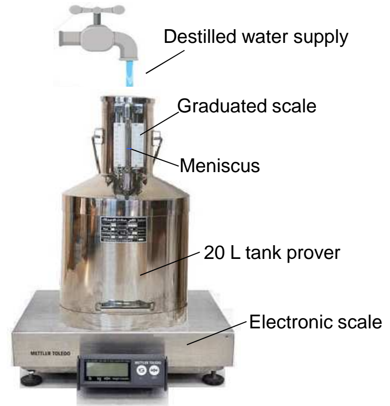
Schematic for calibration of the 20 L tank prover
